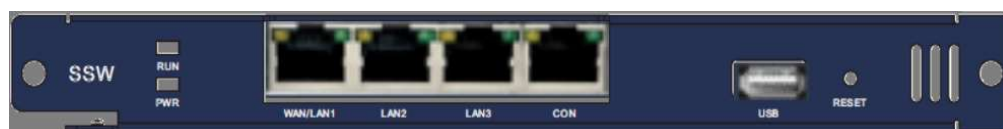
Figure 1-3 SSW system exchange board outlook diagram
